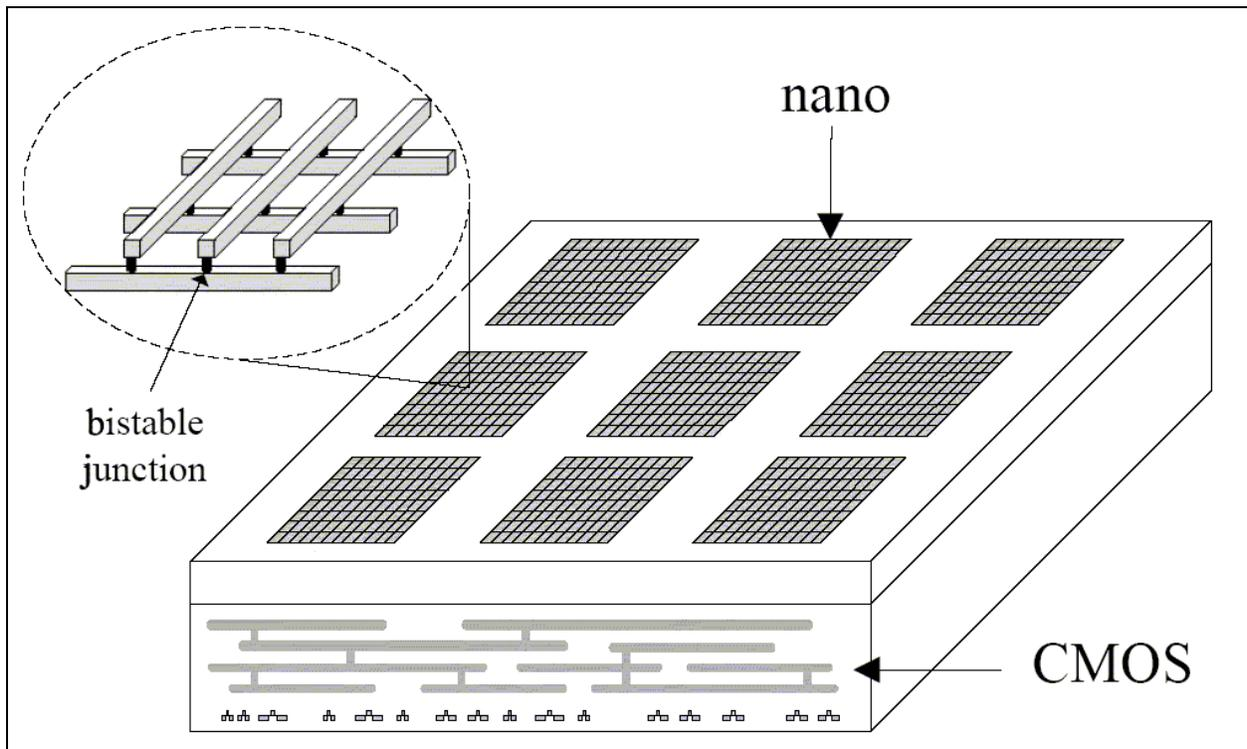
Figure 3. Nanoelectronics on a CMOS IC. (Zeigler & Stan, 2002)
