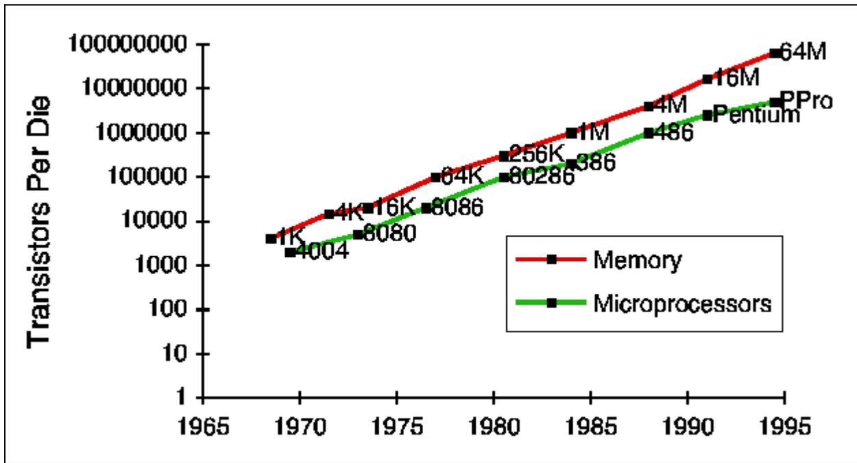
Figure 1. Transistor capacity growth over time. (Lazowska, 1996)
