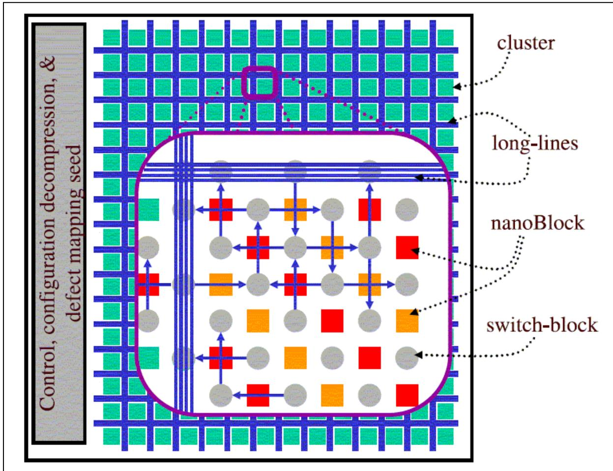
Figure 2. NanoFabric layout. (Butts, DeHon & Goldstein, 2002)
